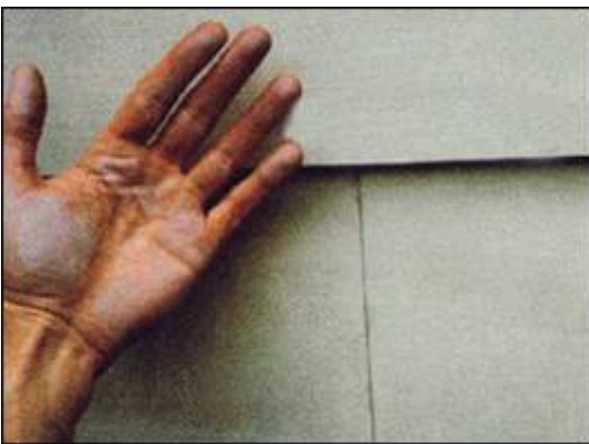
Figure 3: Illustration of the chalking effect
